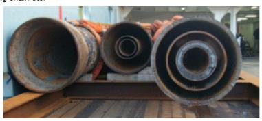
Figure 4-1 - Subsea well casings cut using AWJ based cutting tools, [1]
